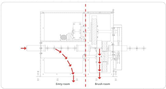
The machine is divided into two chambers:
